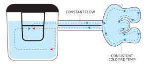
**ICEMAN** with dual pump recirculation technology. The DonJoy<sup>®</sup> IceMan<sup>®</sup> features a recirculation system that allows water warmed after flowing through the cold pad to be preserved and remixed with cooler ice water at a constant flow rate, providing consistent cool water distribution throughout the cold pad.
