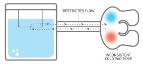
**COMPETITORS** Other versions restrict or pinch water flow to the cold pad, causing variable flow rates and inconsistent cold pad temperatures.
